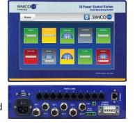
Control Station which shows data for each sensor. It reports the sensor's overall average and individual sensor readings. Sensor attributes such as run time and address are also viewable.
