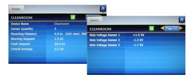
The Control Station also allows for closed-loop feedback adjustments. Closed-loop feedback (CLFB) mode allows the Sensor to directly control output of the neutralizer. CLFB mode offers the most precise static neutralization.
