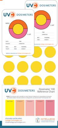
"Most healthcare facilities do not have a means to measure UV-C to determine if effective doses are being delivered. The colorimetric indicators provide an easy means to monitor UV-C dosing."\*
